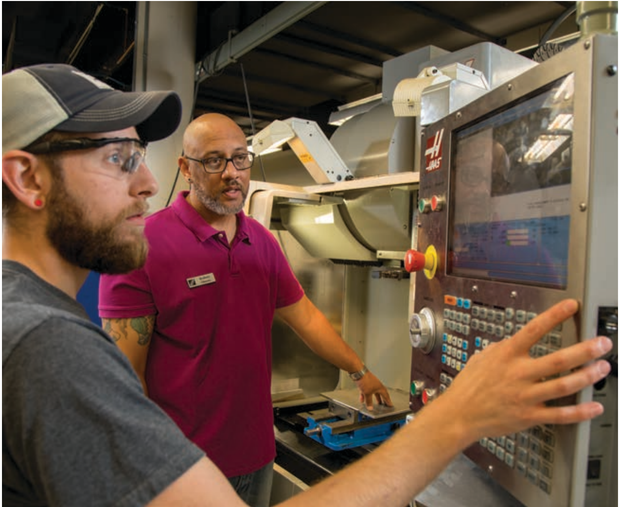
Owens helps Rollogas learn the proper technique for programming one of the lab's computer numeric control (CNC) tools. CNC machines are (literally) cutting-edge tools for advanced manufacturing; they're used for precise cutting, milling and machining.
